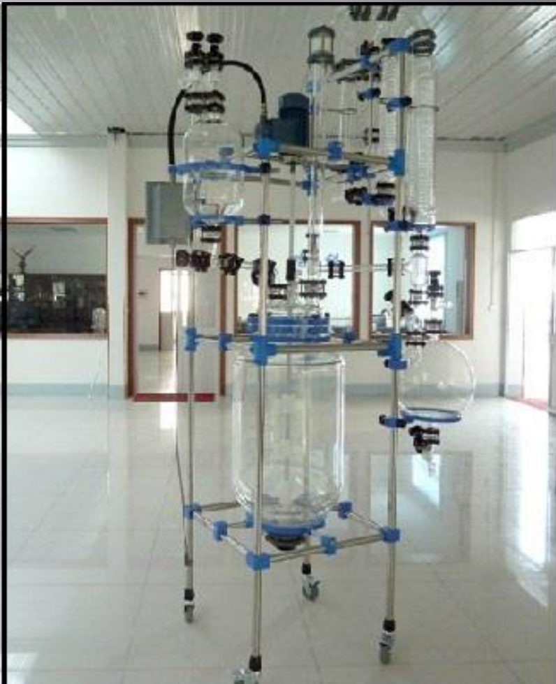
Multifunctional reactor with tail gas absorption device
